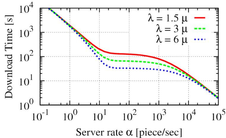
**Figure 1 : Mean download time as a function of the server rate ( $N=100$ ,  $M=2000$ ,  $\mu=0.5$ ).**
