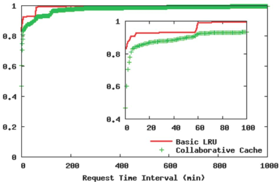
Figure 14 : Cumulative Distribution Function. The y axis is the ration of chunks; the x axis is the time elapsed between two consecutive accesses on a CR.
