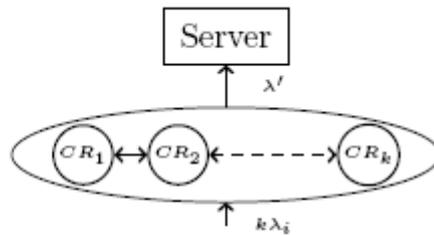
Figure 10 : Cooperative caches connected to a server
